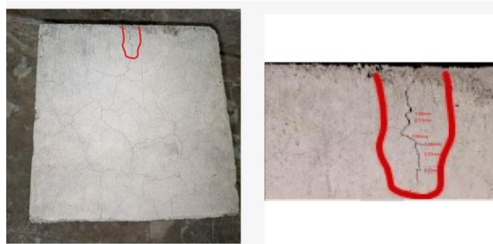
Figure 4.30: surface cracks of 30-CR at 7-day age after heating at 200°C
