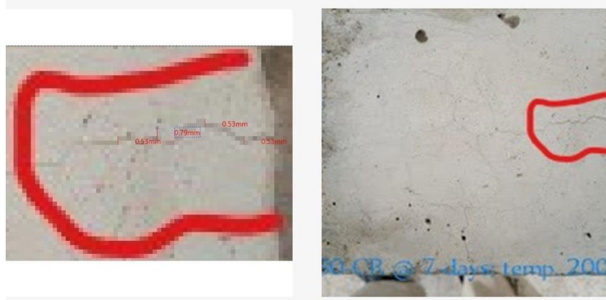
Figure 4.29: surface cracks of 30-CR at 7-day age after heating at 200°C
