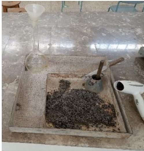
Figure 3.5: Specific gravity of fine aggregates in action
