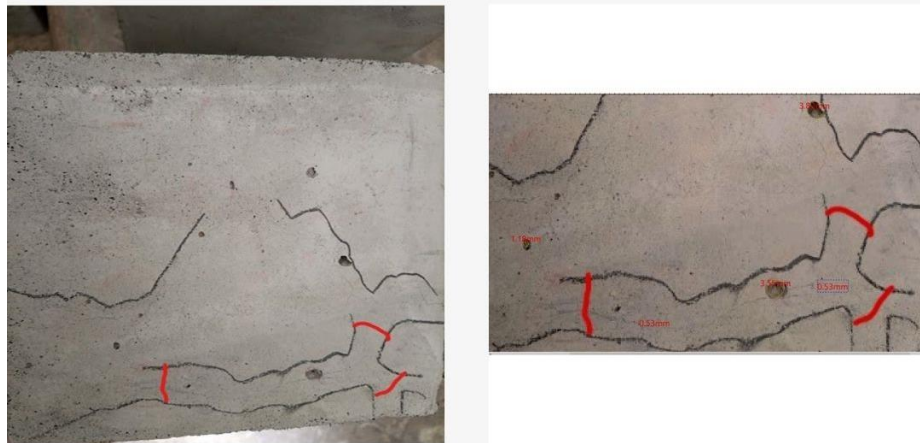
Figure 4.33: surface cracks and pores of 40-CR at 28-day age after heating at 200°C
