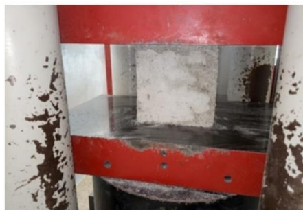
Figure 3.9: 150 mm cube subjected to compression load
