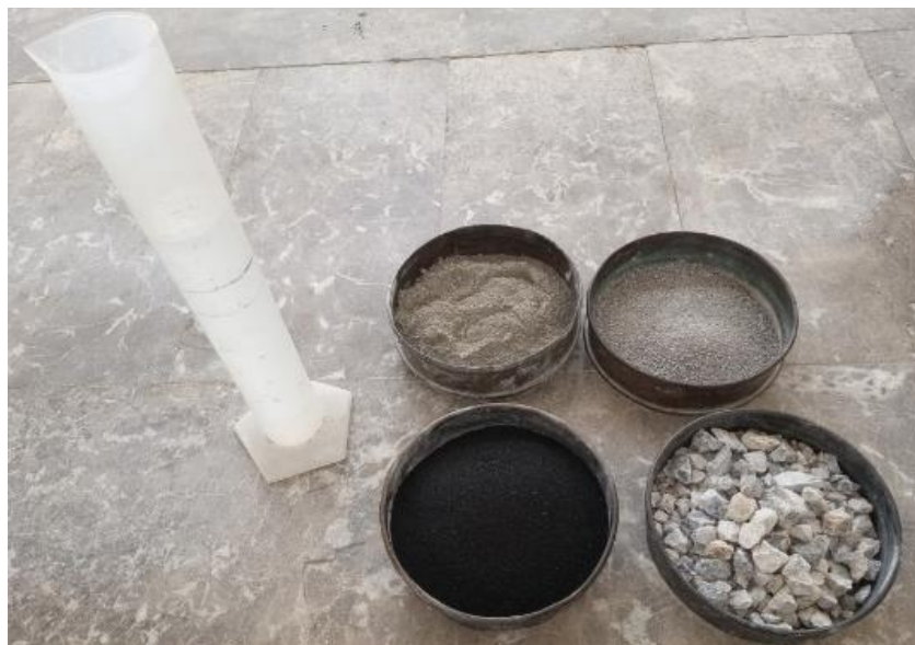
Figure 3.2: Constituent materials of concrete for this research
