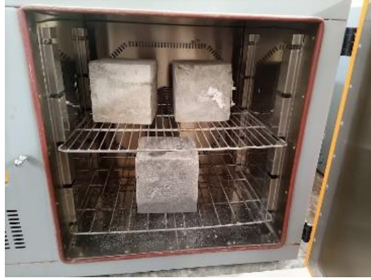
Figure 3.12: Cubes put in oven for degradation
