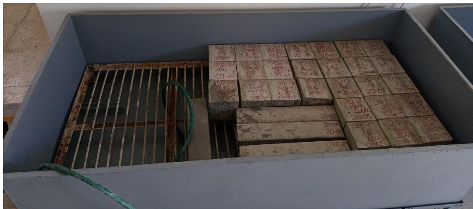
Figure 3.6: Demolded specimens of 20-CR in the tank; inset, tank is being filled with water using hose to start curing
