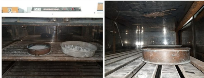
Figure 3.4: Aggregates in the oven for moisture content
