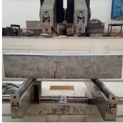
Figure 3.11: beam specimen subjected to flexural load
