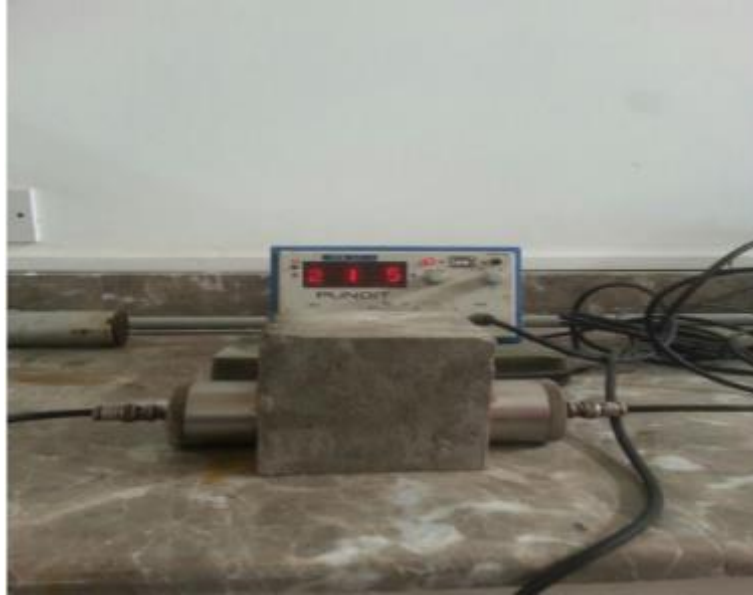
Figure 3.14: Setup of UPV Test Source: (Borghol, 2018)
