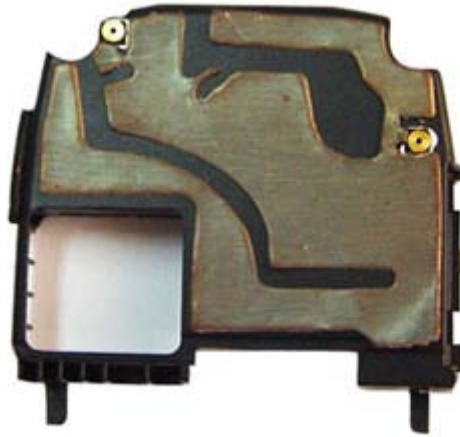
Figure 5: An Internal Cell Phone Antenna.
