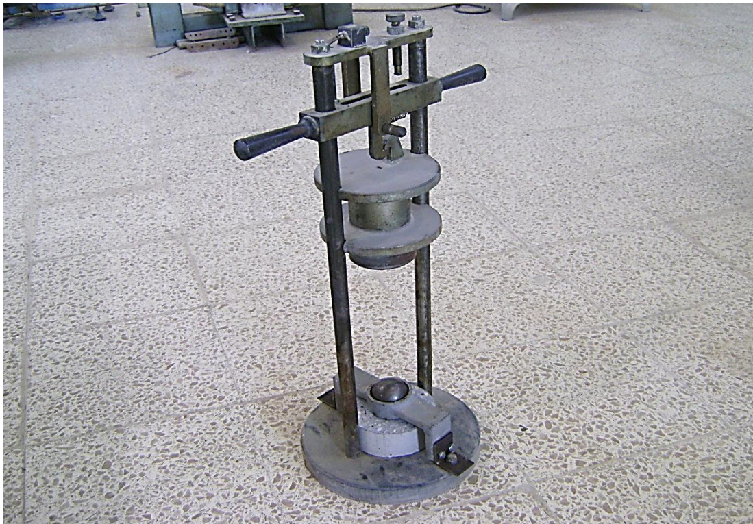
Photo 16: Impact Energy test machine
