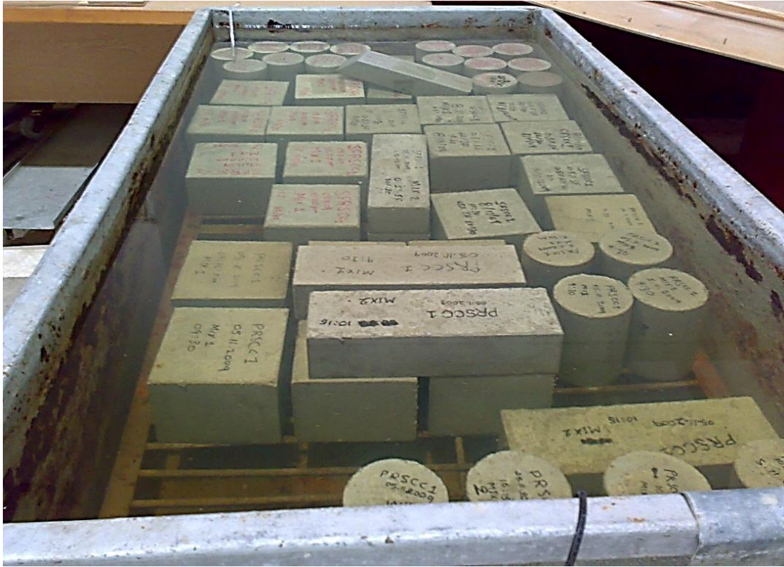
Photo 5: Curing of the specimens within the control tank
