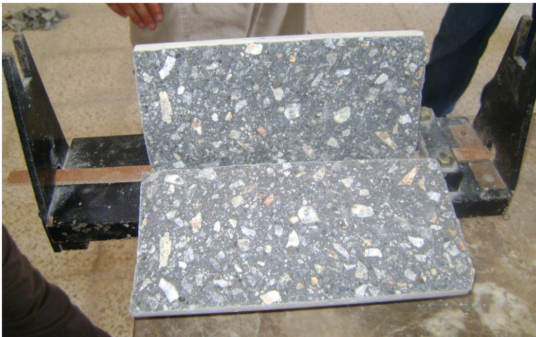
Photo 13: The specimen after Splitting Tensile Strength test
