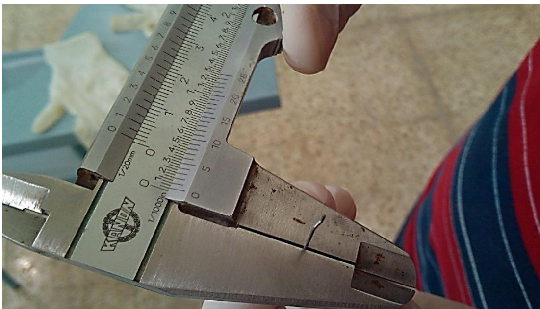
Photo 2: Hooked-end steel fiber with 0.5 mm diameter
