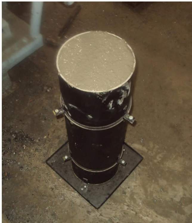
Photo 10: Sample under Column Segregation test
