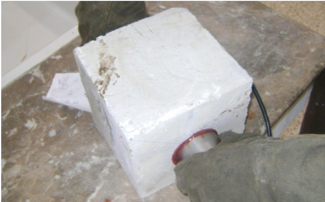
Photo 22: The Pulse Velocity Test
