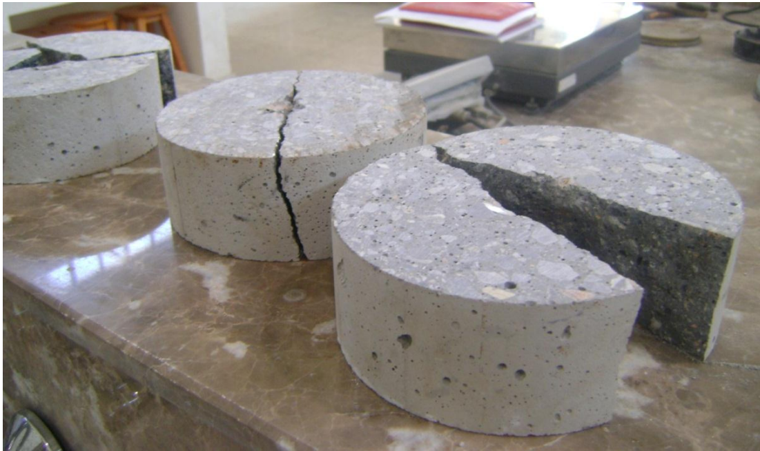
Photo 17: The specimens after failure by Impact Energy Test
