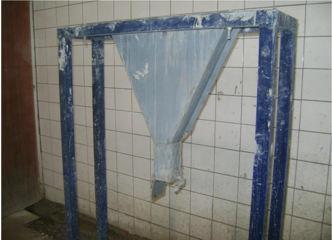
Photo 9: V-funnel test apparatus
