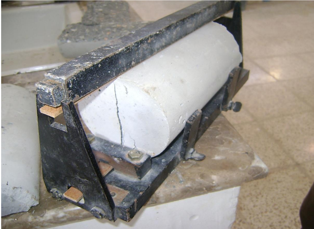
Photo 12: Splitting Tensile Strength test specimen
