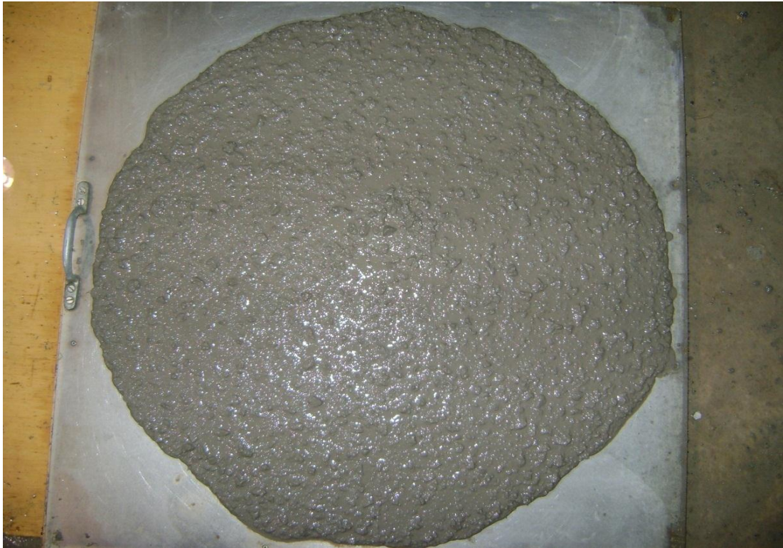
Photo 6: Sample under Slump Flow test
