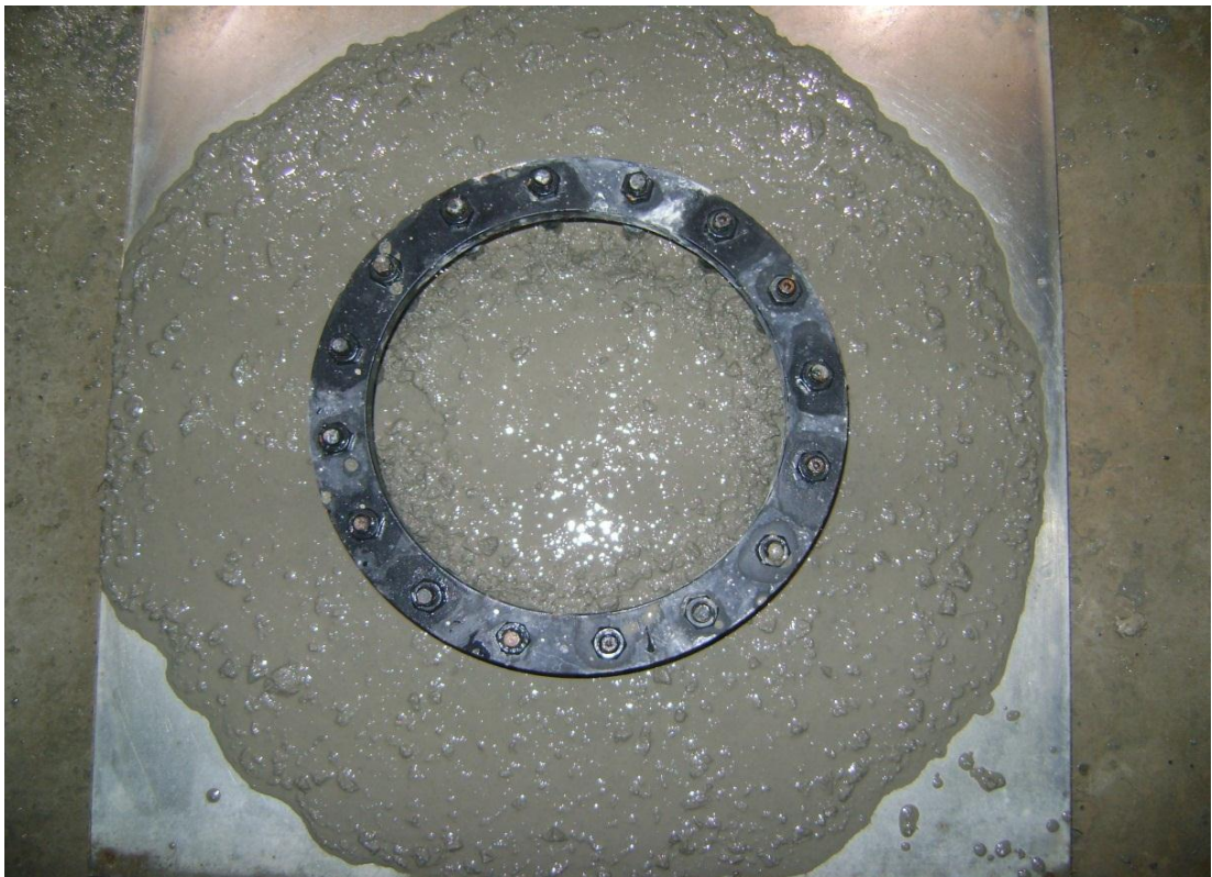
Photo 8: Sample under J-ring test
