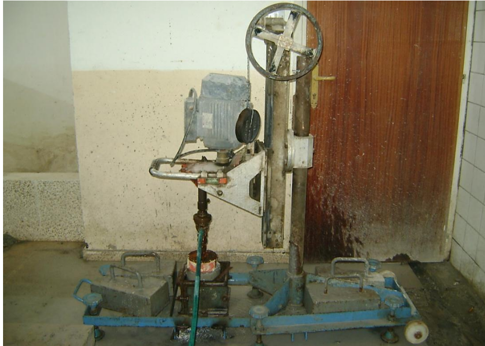
Photo 21: Surface Abrasion Testing apparatus
