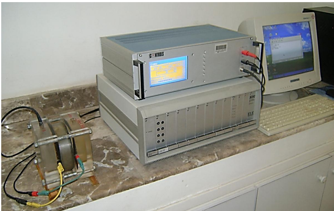
Photo 20: Setup of Chloride Ion Penetration Test
