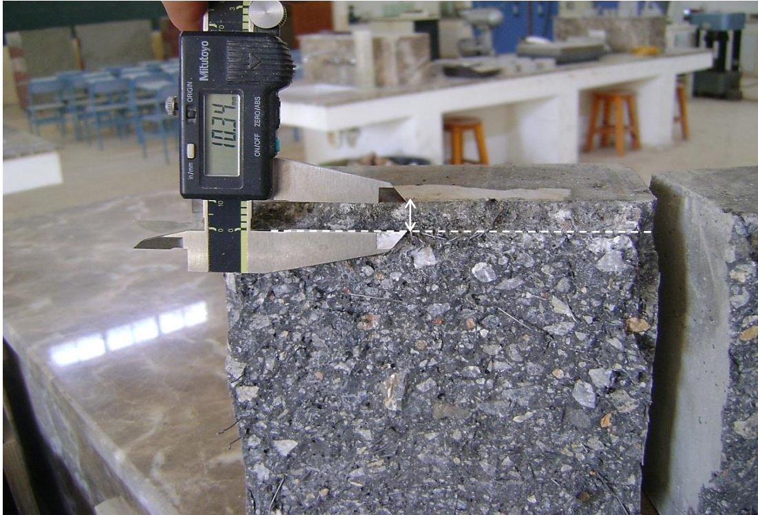
Photo 19: Depth of Water Penetration within the specimen
