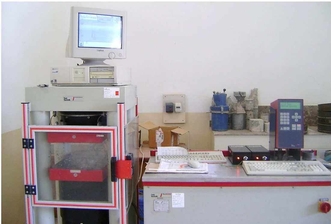
Photo 11: Compressive Strength test machine
