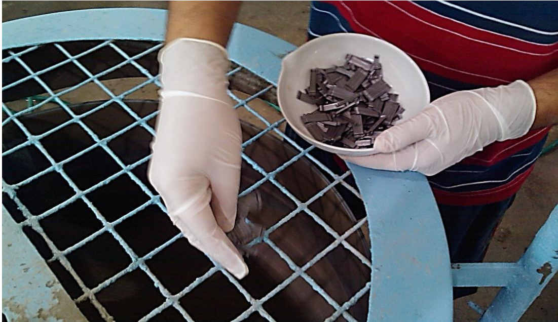
Photo 3: Addition of fibers to the mix from top of the mixer
