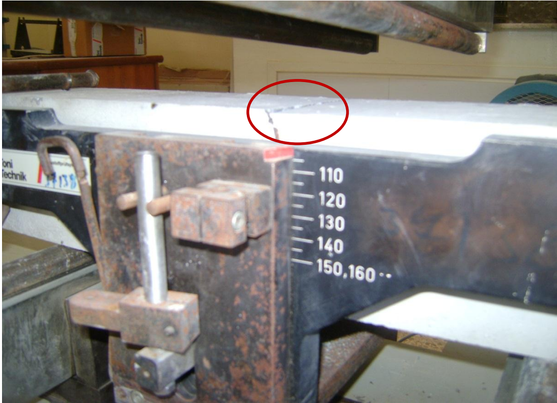
Photo 15: Specimen after failure due to Flexural Strength test
