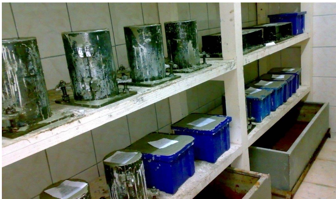
Photo 4: Specimens kept 24 hours in moisture room
