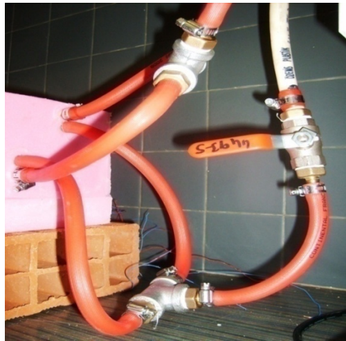
Figure 3.4: Situation of valves.
