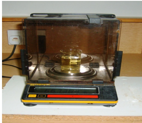
Figure 3.9: Measuring weight of a sample which volume is known to calculate density of the sample
