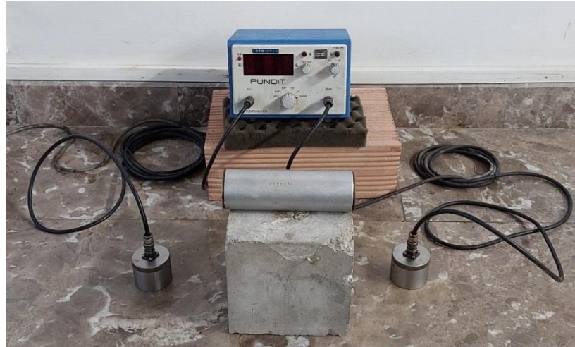
Figure 8: Ultrasonic pulse velocity test apparatus
