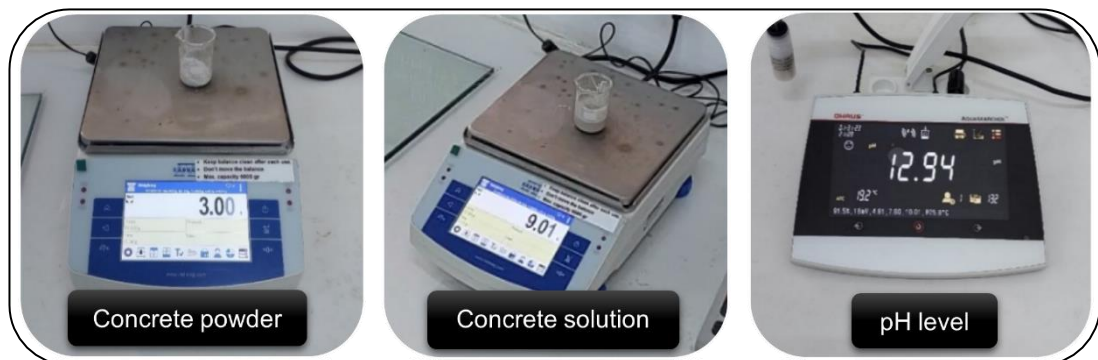
Figure 10: Concrete pH measurement process
