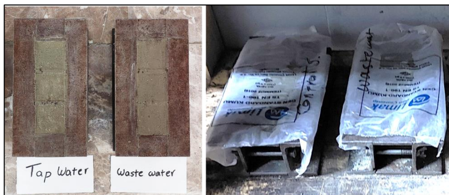
Figure 9: a) Mortar specimen b) Curing condition of mortar specimens
