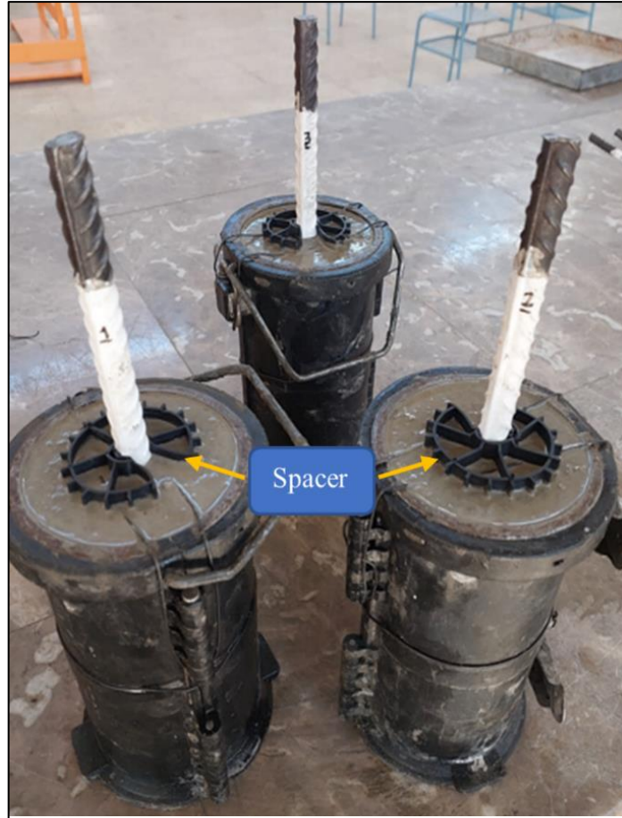
Figure 7: Visual representation of fixed rebars in concrete specimens
