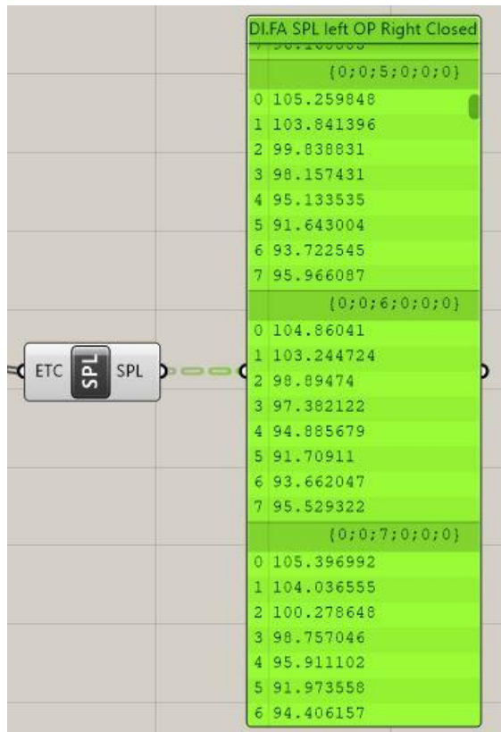
Figure 36. Sound Pressure Level results of Diamond Façade Form when the elements are expanding on the left and contracting on the right (Author, 2023)
