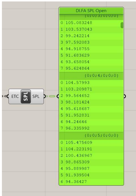
Figure 38. Sound Pressure Level results of Diamond Façade Form when the elements are in total Expansion (Author, 2023)
