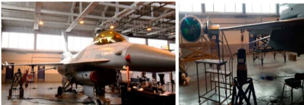
Figure 8: F-16 Ground Vibration Testing Measurement Campaign
