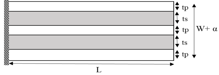
d) Structure 4: 2-layer brass substrate 3 layers PZT-5H
