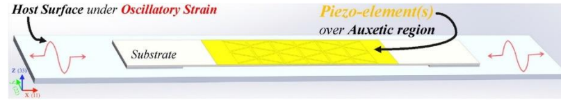
Figure 15: Schematic diagram of APEH bonded on a host structure. A second piezo element can be added on auxetic region underside [37]
