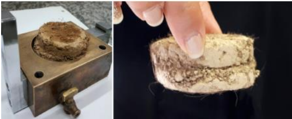
Figure 4: The FHRC sample during the direct shear test's final stage (left) and its integrity's preservation following shear failure (right).
