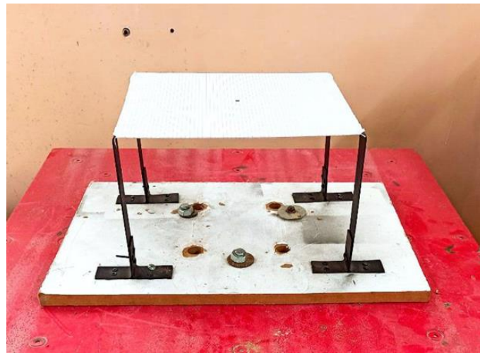
Figure 12: the specimen with checkerboard on the slab for image and video processing tests.
