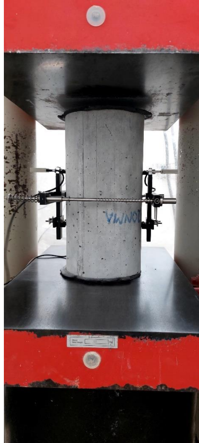
Figure 9: Modulus of elasticity test setup for RCan20NMA
