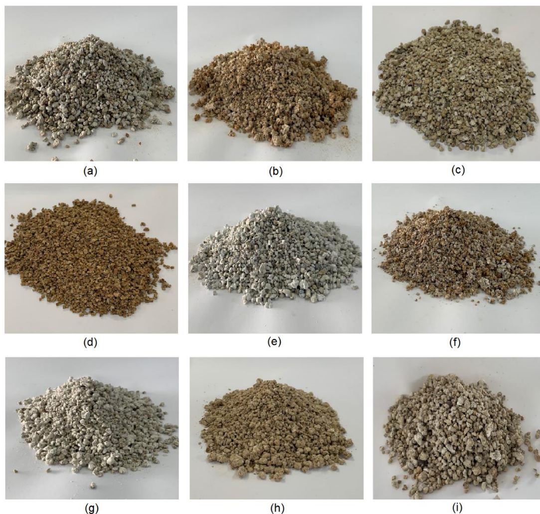
Figure 26: Initial View of the Sorption Materials Before Testing: (a) P-CaCl 2 , (b) V-CaCl 2 , (c) P-LiCl, (d) V-LiCl, (e) P-MgCl 2 (f) V-MgCl 2 , (g) P-LiNO 3 , (h) V-LiNO 3 , and (i) P-CaCl 2 - LiCl.
