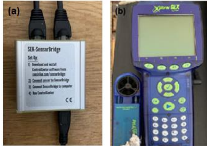
Figure 6: (a) Sensirion SHTC3 Sensor, and (b) Xplorer GLX Weather Anemometer
