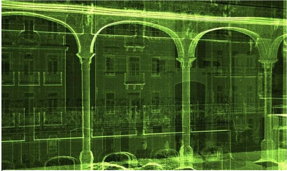
Figure 42: 3D laser scanning of a building facade (URL 15)
