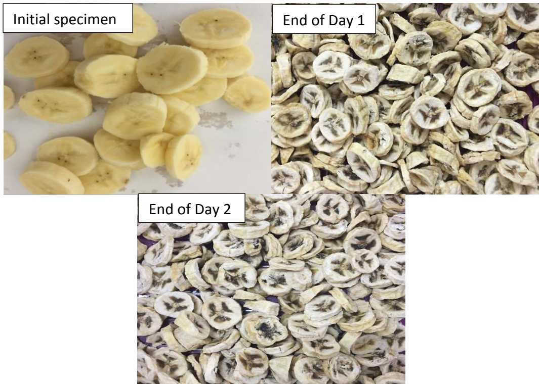
Figure 5.12: Drying sample at the end of each day during banana drying
