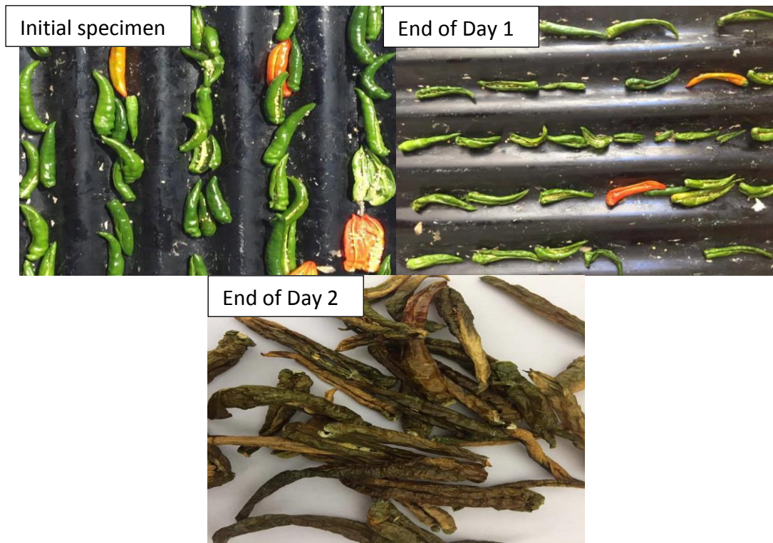
Figure 5.15: Drying sample at the end of each day during chill pepper drying
