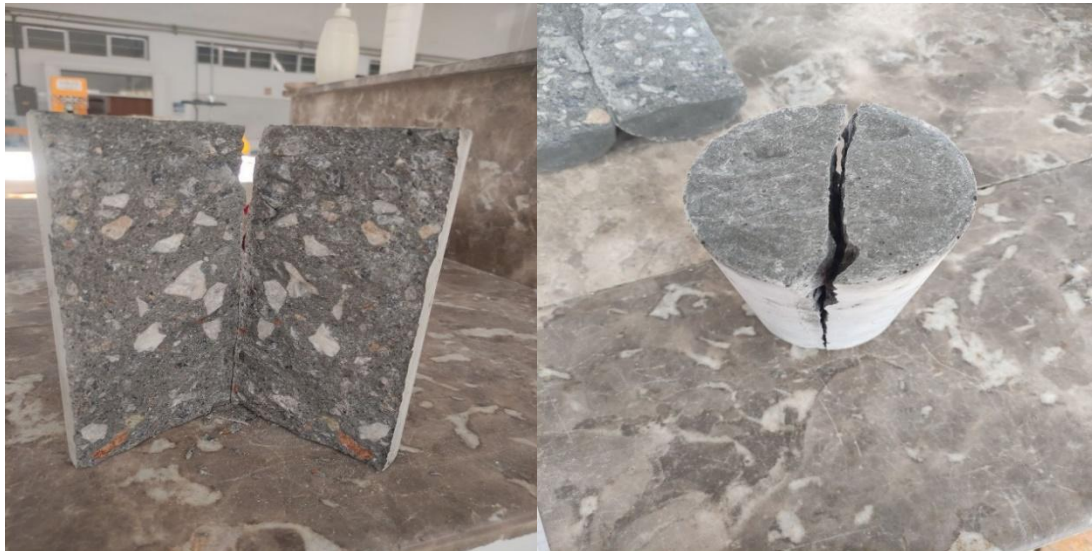
Figure 8: Crushed cylinder sample under axially loading of machine
