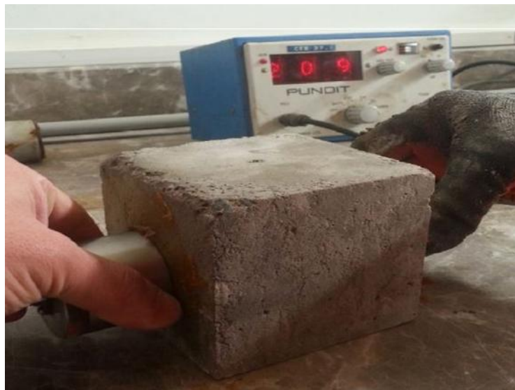
Figure 10: Ultrasonic pulse velocity test of sample
