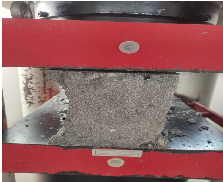
Figure 7: Crushed specimen containing 7.5% SF
