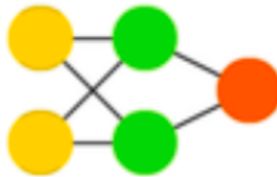
Figure 2.7: Two-layer MLP Processing a 2-Feature Input Vector: 1 Hidden Layer with 2 Neurons (green), and 1 Output Layer with 1 Neurons (red)
