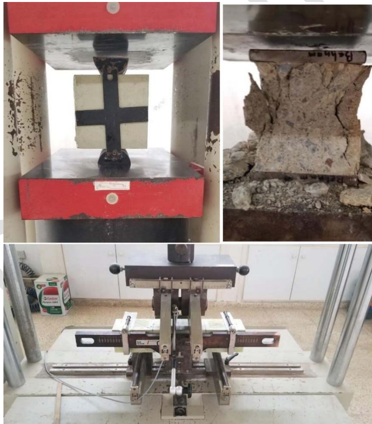
Fig.5 - Experimental setup for evaluating mechanical properties: tensile, compressive, and flexural strength testing
