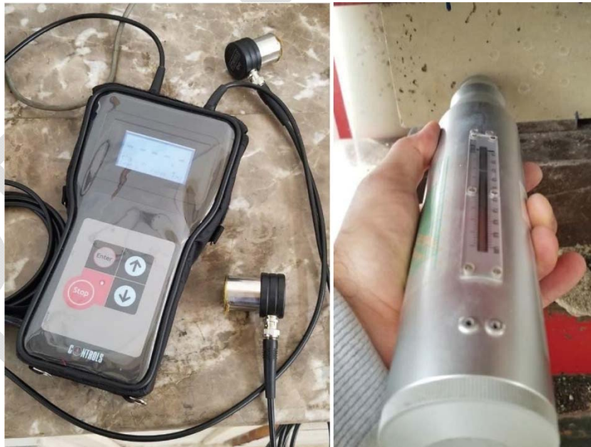
Fig. 6 - Setup for UPV and Schmidt hammer tests on sulfur concrete specimens.
