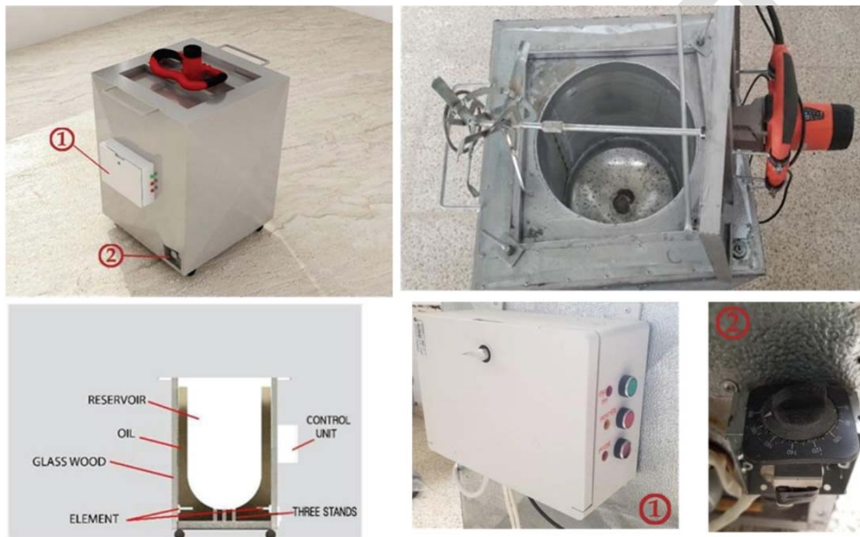
Fig.3 - Custom-built temperature-controlled mixer for sulfur concrete: external view, mixing chamber, control panel, and heating system layout.
