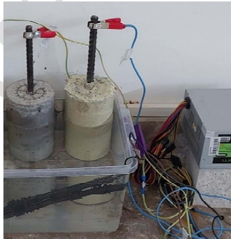
Fig.9 - Setup of accelerated corrosion test using partially immersed specimens and DC power supply.
