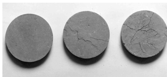
FIGURE 1: Compacted soil samples showing increase in macropores after cyclic drying
