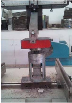
Fig. 1 Compressive strength test.
