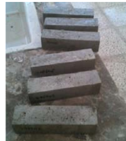
Fig. 5 Samples of flexural strength test prisms.
