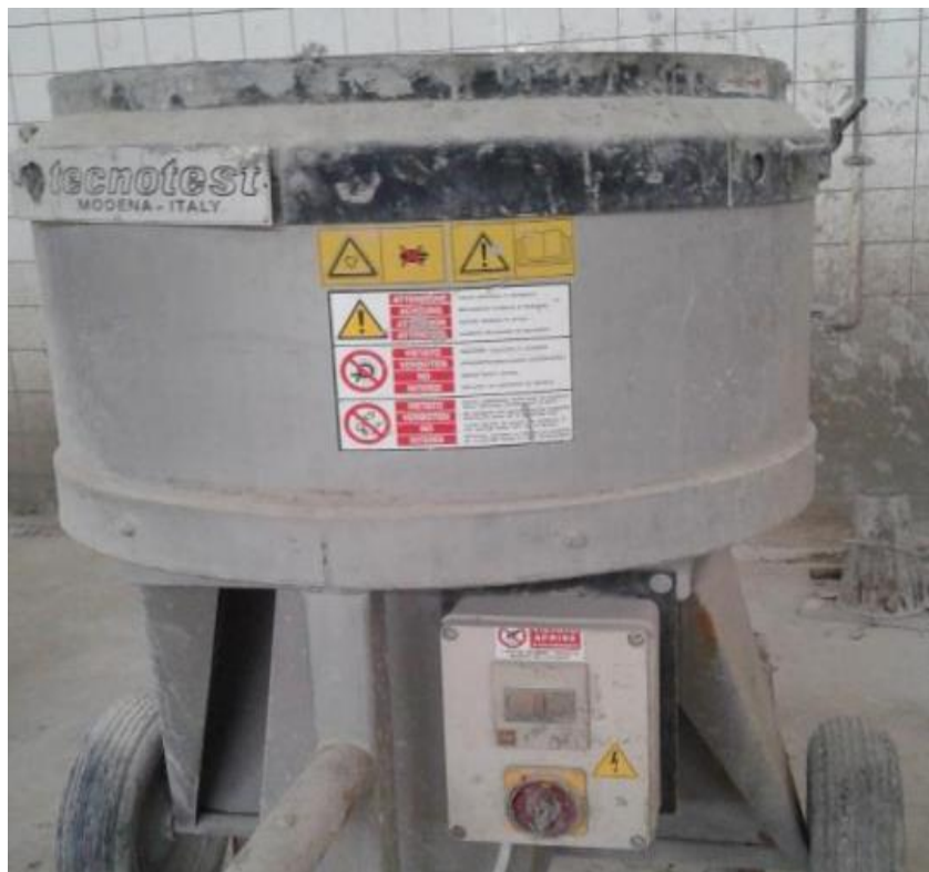
Figure 11: Concrete mixer with capacity of 0.25 cubic meter
