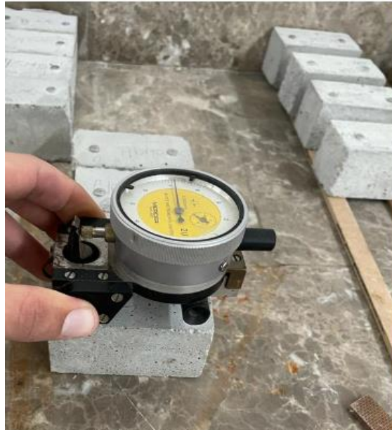
Figure 23: Measuring drying shrinkage
