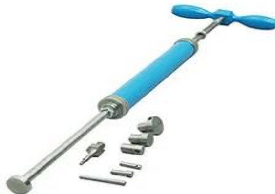
Figure 17: Concrete and mortar penetrometer
